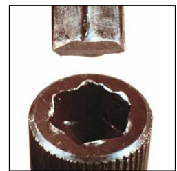
Tool and fastener damage is common
