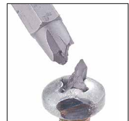
Concentrated stresses can cause breakage
