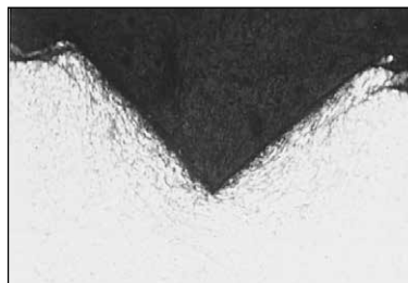
Mag-Form® Thread Forming Fasteners Compressive action forms strong threads in low-ductile materials
