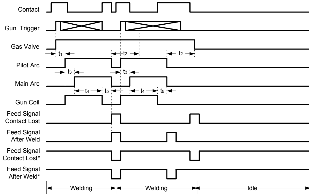
Starting a weld during gas postflow
