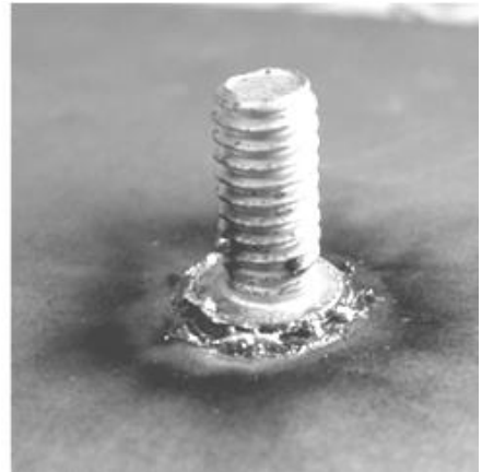
Situation: Hot Weld
