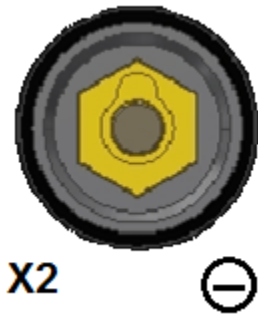
Figure 1.4 Gun Welding Cable Socket
