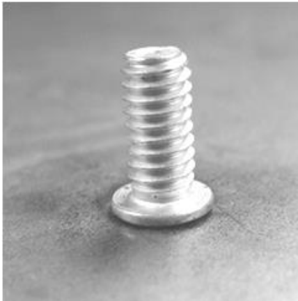
Situation: Cold Weld
